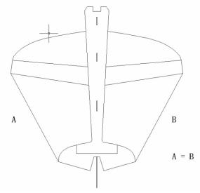
**Step11.**Glue the side board and main board of fuselage.
