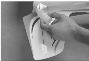
**Step 12.**Hinge the rudder to the back of the fuselage, using the same techniques that you used tohinge the Elevator to the stabilizer.
