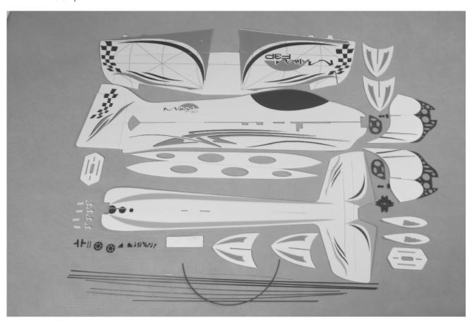
Fuselage main board - 1 Wing with Ailerons - 1 Horizontal Elevator - 1 Rudder - 1 Wing Fences - 4 Landing Gear Struts - 2 Doublers with Round Hole - 2 Wheel Covers - 2 Main Gear Wheels - 2 Carbon Fiber Rods 1.3mm - 5 Carbon Fiber Rods 2.0mm - 1 Doublers with Elongated Hole -2 Plywood Pushrod Supports - 2 Plain Wires - 1 Control Horn Backplates - 4 Control Horns - 4 Carbon Fiber Strips -3 Heat-Shrink Tubing - 1 Wood Screws - 4
