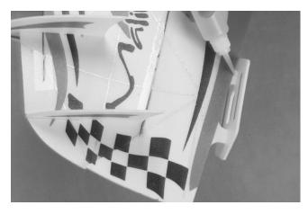
Mount your ESC to the fuselage side, using a piece of double-side foamtape (not included).
