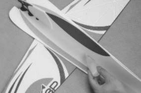
Glue the side board and main board of fuselage. Make sure the side board is vertical to the main board.
