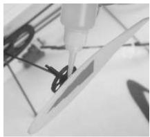
Install wheel covers on the chock beside the wheel. Screw one more chock outside of the cover,glue it.
