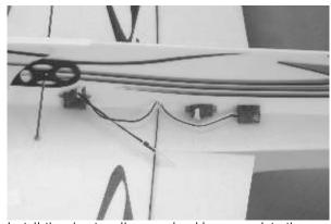
Install the elevator aileron and rudder servos into the servo mounting hole in the right side of the fuselage. Use a dab of foam-friendly thick C/A to secure them into place. Because the size of servos differs, you may need to cut the servo mounting hole larger to fit your particular servos.
