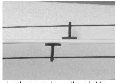
Slide one plywood pushrod supports over the end of the carbon fiber rod and temporarily push the plywood pushrod supports into the one precut slots in the fuselage.
