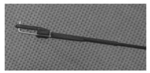
Secure one piece of wire to one end of the carbon fiber rod, using one piece of heat-shrink material. The piece of wire should overlap the carbon fiber rod at least 1" (25mm). Heat the heat-shrink material with a heat gun to shrink it into place. PRO TIP For extra security, apply a few drops of foam-friendly thin C/Ato the end of the pushrod and allow it to "wick" into the joint.
