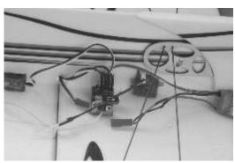
Plug the servo and ESC leads into their proper slots in your receiver, then mount your receiver to the side of the fuselage, opposite the ESC, using a piece of double-sided foam tape (not included). Run the antenna out the bottom of the fuselage and secure it along its length, using pieces of clear tape (not included). Do not cut the antenna shorter. Allow the excess to hang beyond the back of the fuselage.
