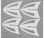
Glue four wing fences to the wing, making sure that the back edge of each wing fence is even with the aileron hinge line. Use a builder's triangle to make sure that the wing fences are perpendicular to the wing.
