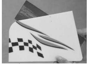
Sand a 45° bevel into the left side of the leading edge of the rudder.
