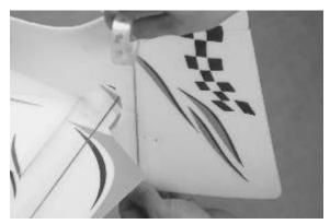
Hinge the rudder to the back of the fuselage, using the same techniques that you used to hinge the Elevator to the stabilizer.
