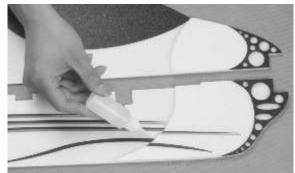
Glue the foam strengthen slice to the head of fuselage side board.
