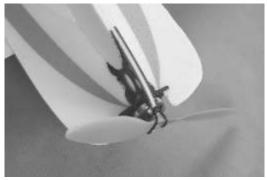
Install the propeller and decals. Balance your propeller, then install it onto your motor. Using a clean cloth, wipe the airframe down completely to remove any dust, debris and oil.
