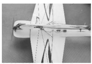
Install the wing bracing is similar to installing the fuselage bracing, as you want the rods to be glued to the carbon bracing that has been preinstalled on the wing and fuselage. The rods are staggered and fit into notches in the fuselage. Make sure the rods are straight and are not flexing the wing. The wing should be flat and parallel to the horizontal stabilizer, while also being perpendicular to the vertical fuselage.
