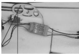
Mount your ESC to the fuselage side, using a piece of double-side foamtape (not included).
