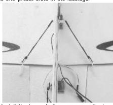
Install the horn of aileron same as the horn of stabilizer.
