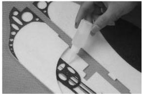
Glue the landing gear reinforcement to the fuselage side board.
