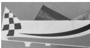
While holding the elevator tight against the stabilizer, apply a strip of clear plastic tape (not included) to the top of the hinge line on the elevator.
