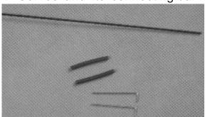
Cut two pieces of carbon fiber rod ,then cut two pieces of heat-shrink tubing to a length of 1-1/2" (38mm). Cut two pieces of plain wire to a length of 1-1/2" (38mm), then make a L-Bend in one end of each piece of wire and a 4mm long 90° bend in the other end of each piece of wire.
