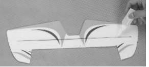
Cut a piece of carbon fiber strip to a length of 14-2/3" (376mm), then glue it to the below of the elevator, using some foam-friendly C/A. Make sure the elevator is flat and the leading edge is straight while the glue cures.
