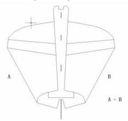
Glue the wings with aileron to fuselage. Notice: Measure from the tips of the wing to the rear of the fuselage. The measurements must match from right to left. If not, adjust the position of the wing until both measurements are equal.
