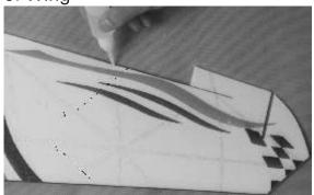
Use foam-friendly C/A to glue the carbon strips to A and B to strengthen the wings.
