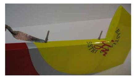
$\Box$  step 7 Always with 5 minutes epoxy glue the hinges in the fuselage. If necessary clean the zone of the hinges with paper towels and rubbing alcohol.
