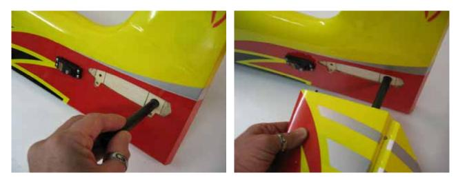
$\Box\Box$  step 5 Fix the stabilizer on the fuselage with the provided 3mm screws and washers.
