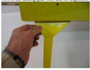
□□ **step 7**Once satisfied with the fit, glue the fillet on the landing gear using medium CA. Use the glue carefully avoid over runs on other areas.
