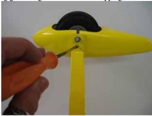
□□ **step 6**Test fit the landing gear fillet and his alignment.
