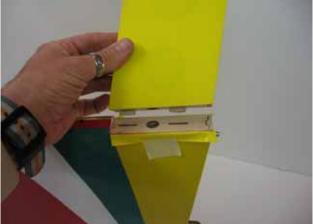
□□ **step 5**Use the covering iron carefully, at a medium temperature, to glue the cover material down around the area of the fillet. Use caution while working around areas where the cover material overlaps to prevent separating the covers.
