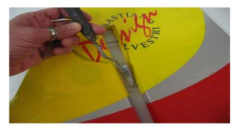
$\square$  step 8 Work the rudder right and left some times to work the hinges and check for proper movement.
