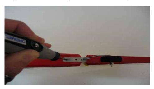
$\square$  step 10 Use the two self-tapping screws to fix the tail wheel as follow.
