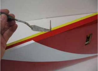
□□ **step 3** Carefully glue, with 5 minutes epoxy, the hinges into the aileron.
