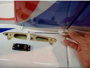
$\Box\Box$  step 2 Locate the new elevator and verify, placing the three hinges in their holes, the correct position and alignment of the elevator with the stabilizer panel.
