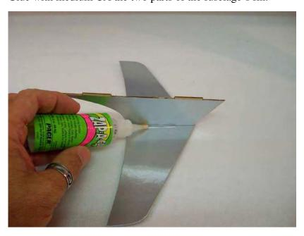
$\Box$  step 3 With the hobby knife open the two slots on top fuselage and carefully glue the fin with medium CA.
