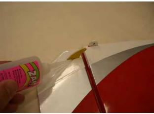
□□ **step 4**Locate the servo into stabilizer in his location, bringing out the servo's lead.
