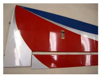
□□ **step 2** Carefully glue, with some drops of thin CA, each of the four hinges in the aileron.
