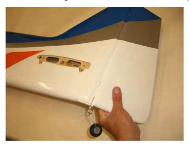
$\Box$  step 8 Using a 1,5mm drill bit, carefully drill the two holes for fixing the tail wheel on the fuselage. Use the two self-tapping screws to install the tail wheel as follow.
