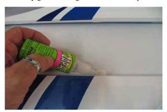
$\Box\Box$  step 3 Locate the elevator hinges into the stabiliser. Glue carefully the hinges in the stabiliser with some drops of thin CA.
