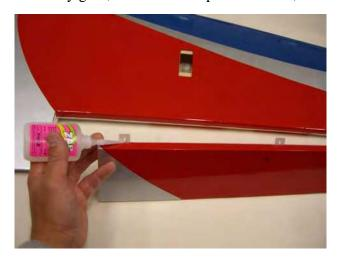
□□ **step 3**Locate the aileron and carefully glue, with some drops of thin CA, the hinges into the wing panel.
