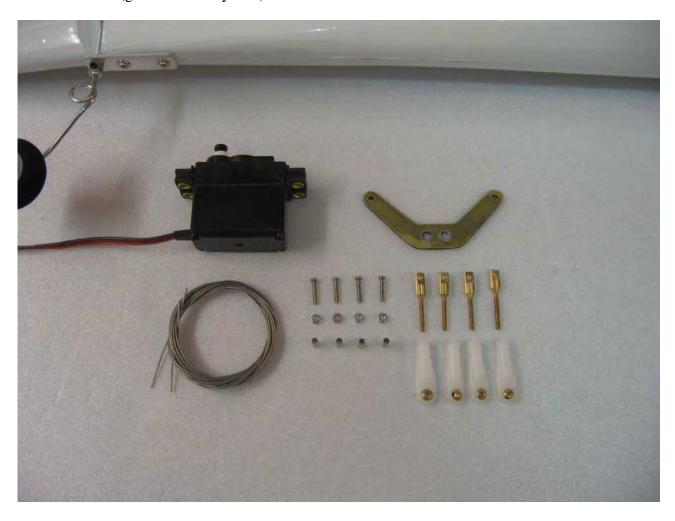
$\square$  step 2 Drill the location for the four self-tapping screw using a 1.5mm drill bit and install the servo as per the picture.
