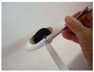
□□ **step 6**Hold the wheel pant parallel to the fuselage and drill the location for the wheel pant screw using a 1,5mm drill bit. Attach the wheel pant to the landing gear using a 2mm short self-tapping screw.
