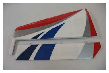
□□ **step 2** Carefully glue the hinges, with some drops of thin CA, in the elevator only.
