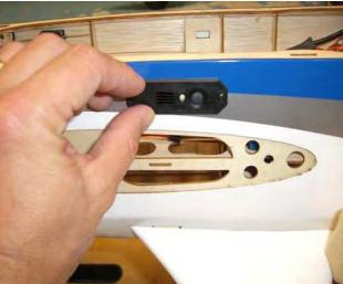
$\square$  step 2 Locate and install the switch with a Phillips screwdriver as follow.
