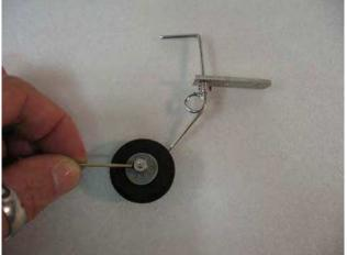
$\Box$  step 3 With the hobby knife cut a groove 20mm length into the rudder. Using a 2mm drill bit, carefully drill the hole into rudder, 20mm from the base level, for the tail wheel, as follow.
