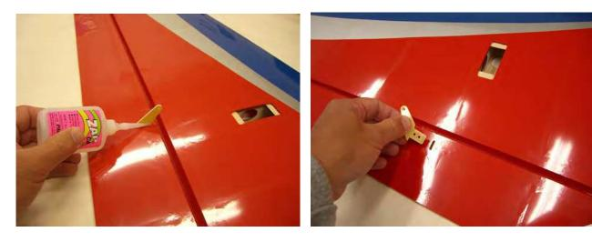
$\Box\Box$  step 4 Drill the location for the four self-tapping screw using a 1.5mm drill bit and install the servo into the wing panel using a Phillips screwdriver, as per the picture.
