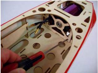
□ **step 5**Apply the velkro on the ESC location.
