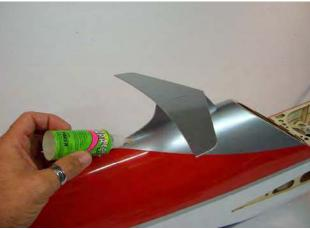
□□ **step 4**With the hobby knife open the slot on the wing's leading edge and test fit the fin on wing panel.
