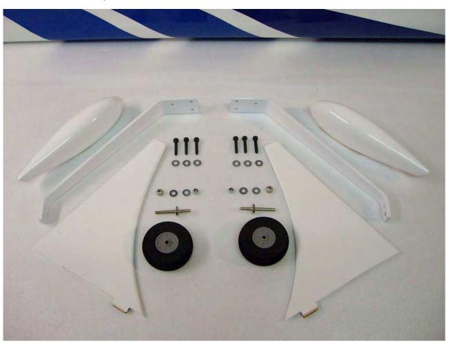
$\square\square$  step 2 Using screws and washers, install the landing gear as follow.
