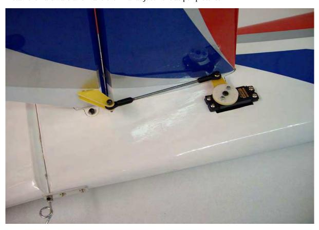
$\Box$  step 14 When you like to install again the F3A elevators, remove the 3D elevator with control horns and servo arms and the carbon tube, as follow.
