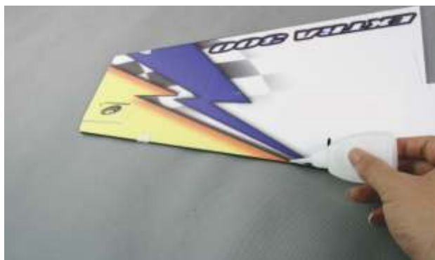
3. Paste the corresponding carbon strip on wing with adhesive tape (as picture shown), then glue it well.
