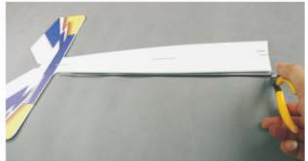
13. Cut out rudder from fuselage.
