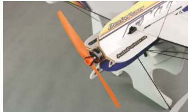
88.Assemble prop on the motor and fix it well via O-shaped ring.
