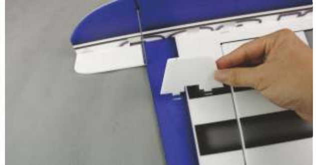
27.Insert carbon rods Supporter into the related slot of wing as picture.
