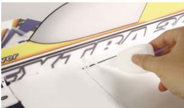
53. Insert aileron control horn into the reserved slot of aileron, and glue it well.
