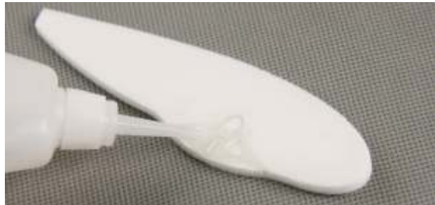
24. Fix wheel stopper reinforcement on wheel cover with glue.
