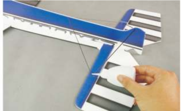
36.Connect #13 carbon rod as picture, then glue it well.
