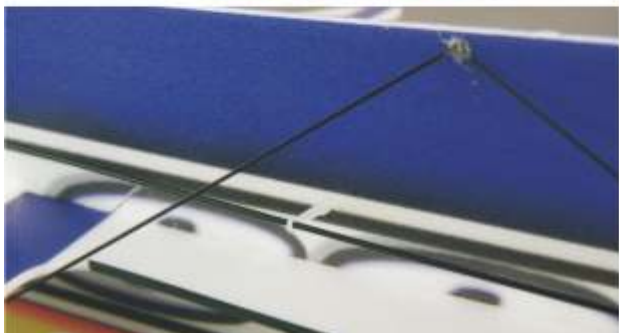
70.Assemble push-pull rods as picture, and glue them well.
