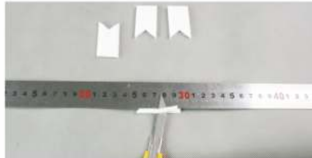
46. Cut one 45 degree bevel angle on both sides of reinforce plates. (left side and right side)
