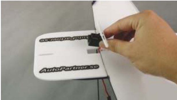
39. Put aileron servo into the slot as picture.
