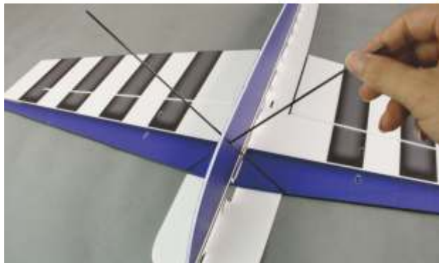
23.Insert carbon rods into corresponding hole on fuselage.
