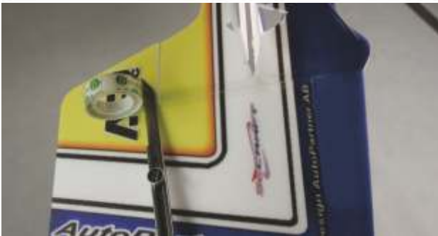
43. Connect rudder with fuselage tail. (Ensure 1mm between the connect face).
