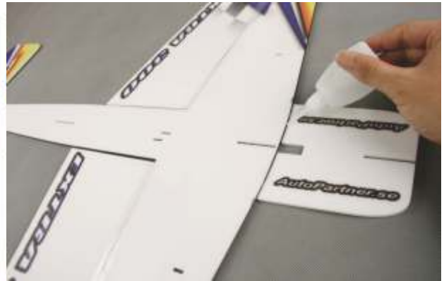
19. Connect horizontal fuselage and wing with glue.
