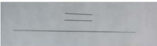
61. Cut out #12 carbon rods to the suitable length as rudder and aileron push-pull rod.
