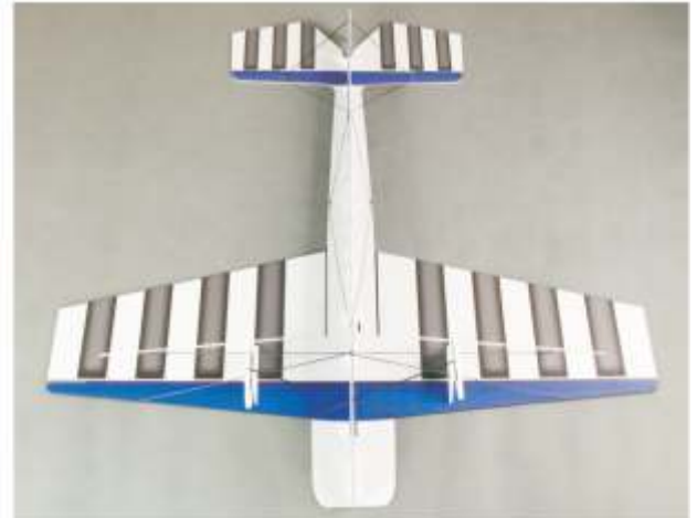
37. Carbon Rods reinforcing in the middle of fuselage.
