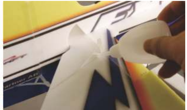
54. Insert two-way control horn into the reserved slot of stabilizer, then glue it well. (Ensure it is in the middle).
