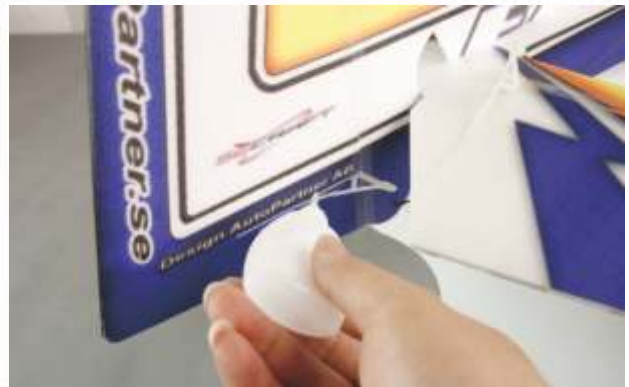
55. Insert one-way control horn into the reserved slot of rudder, and glue it well.
