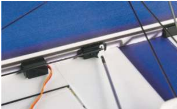
69.Insert rudder push-pull rod with Z end into the hole of rudder servo arm, and fix the arm on servo via screws.
