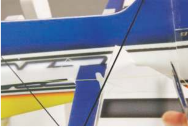
75. Cut 2pcs of string, make they 6-8cm longer than the length from stabilizer servo to its control horn.
