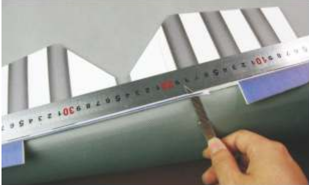
10. Cut a 45 degree bevel angle on elevator.
