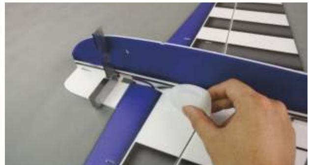
21. Insert lower vertical fuselage into the slots on horizontal fuselage, then fix them with glue. Make sure they're perpendicular to each other.
