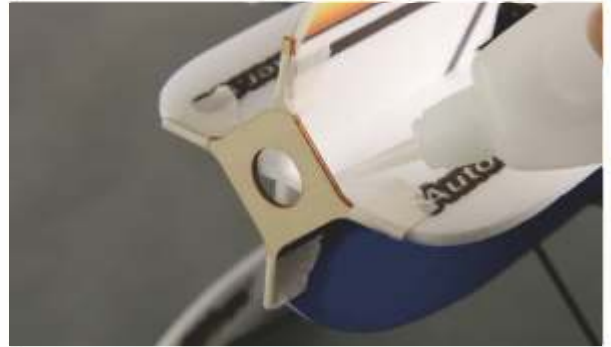
45. Paste motor mount onto plane nose, then glue it well as picture.
