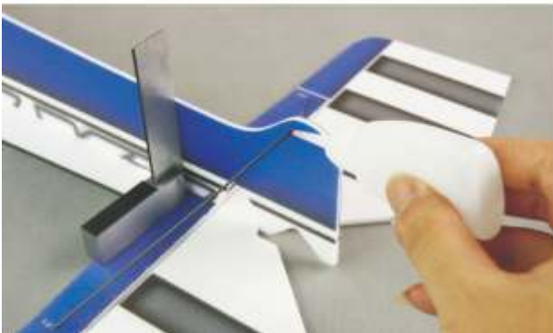
35.Insert carbon rods into the related holes on fuselage tail and stabilizer, and glue them well. (Ensure fuselage with horizontal fuselage be at vertical.)
