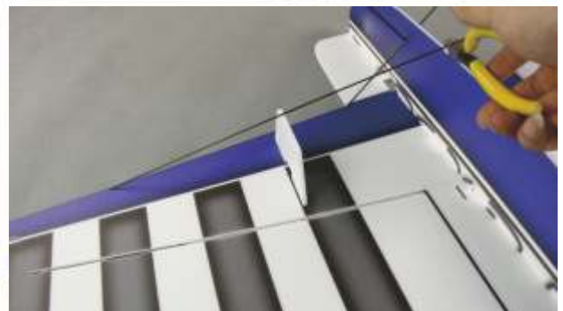
31.Insert #12 carbon rod (850*Φ1.5 MM) into the slot of wing, and through the slot of carbon rod supporter, then cut it off when it reach lower fuselage. As picture.
