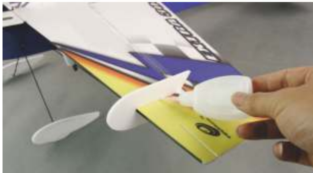
50. Insert wing fence into wing and glue it well.
