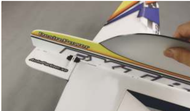
42. Put upper fuselage into the slot of horizontal fuselage, and glue it well. (ensure upper fuselage is vertical with horizontal fuselage.)
