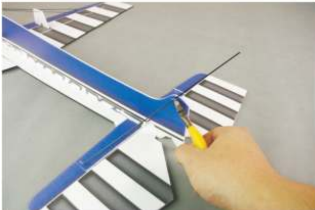
34.Insert #12 carbon rod into the 3rd hole on stabilizer (from back to front), and cut it off when it reach lower fuselage. As picture.
