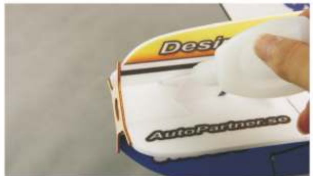
47. Glue reinforce plates on motor mount and nose as picture.
