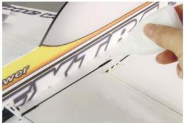
65. Insert connected push-pull rod with Z end into the hole of rocker arm, and the other end into the hole of aileron control horn. Then glue them well.
