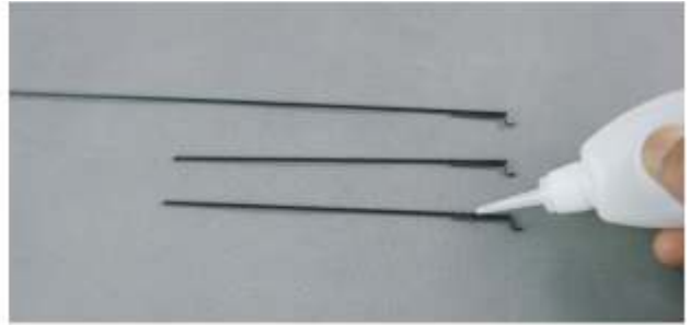
63. Connect push-pull rods with heat-shrink tube and Z-shaped wire, and glue them well.
