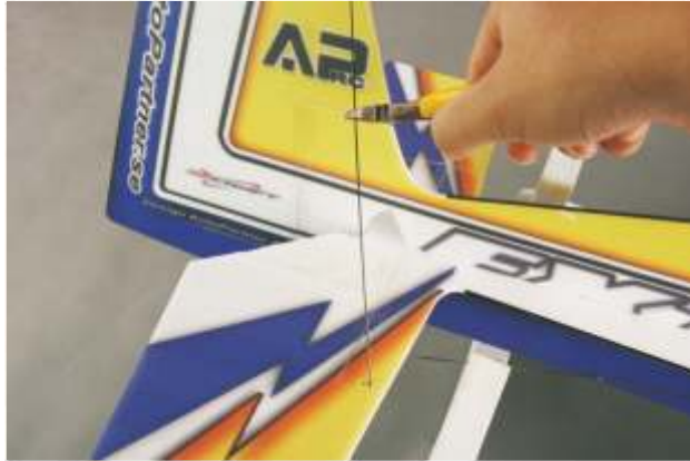
84.Insert the remainder carbon rod of #13 (850*Φ1 MM) into the slot of stabilizer, cut off the other end according to the hole of upper fuselage.
