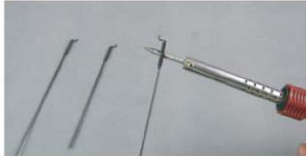
64. Fix the connected push-pull rods via searing iron.
