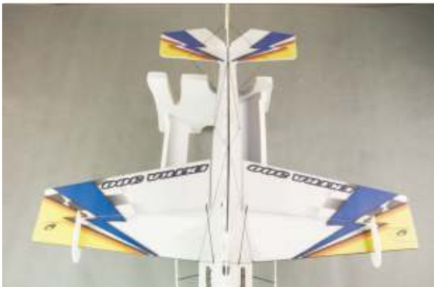
86.Cut remainder reinforce carbon rods to be suitable length, and reinforce upper fuselage. (Ensure these reinforce rods will not disturb stabilizer string and aileron push-pull rods.)
