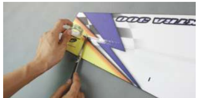
7. Connect aileron with wing together by adhesive tape (keep 1mm clearance between the connection).
