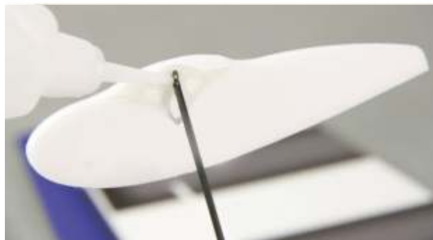
25. Connect wheel stopper with carbon rod as picture, then glue it well.
