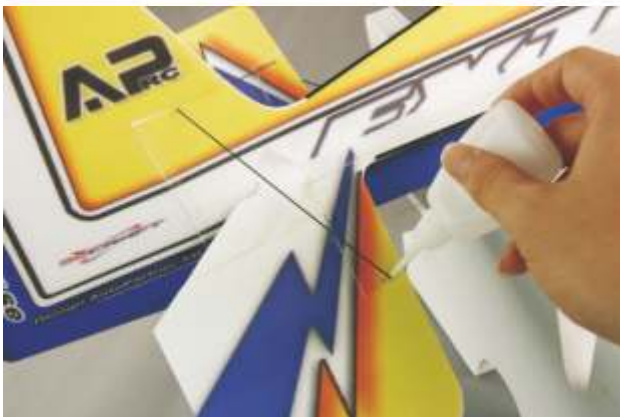
85.Insert one end of reinforce carbon rod into the hole of stabilizer, the other end into hole of fuselage, then glue them well. (Them same as the other side.)
