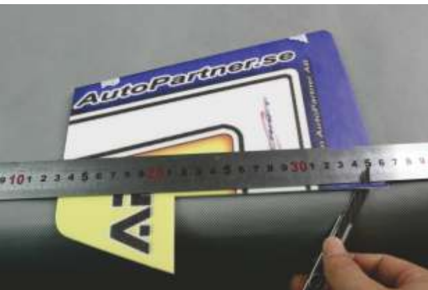
18. Cut a 45 degree bevel angle as picture shown.
