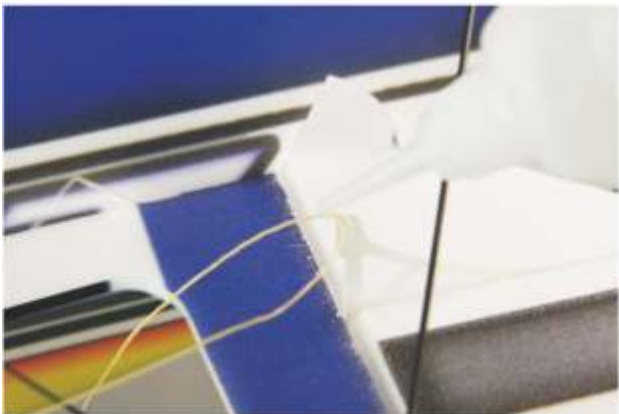
77. Pass one end of string through the hole of stabilizer control horn, tie a knot, then glue it well.
