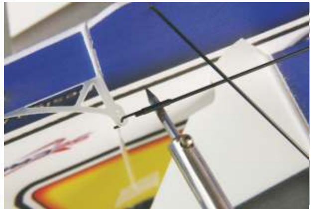
72.Fix the connected push-pull rod with Z-shaped wire via searing iron.
