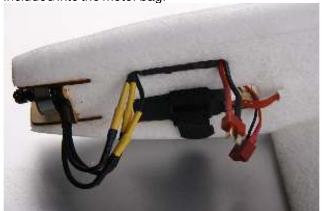
23. Install the ESC into the pre-cut slot of the fuselage, install the battery pack into the next slot of the ESC by using the velcro.
