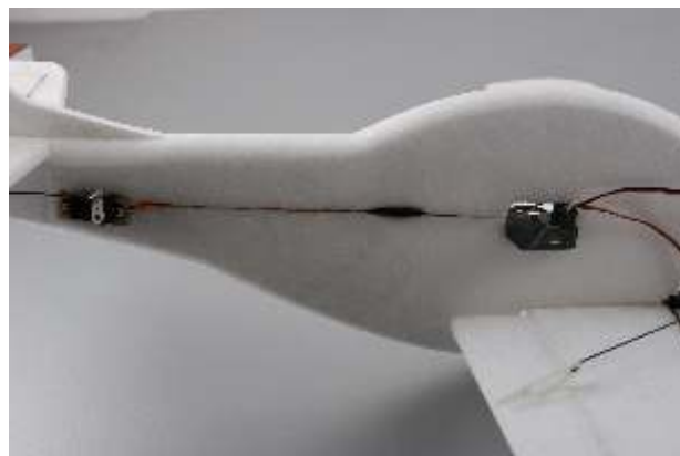
26. On the side of the fuselage , pls cut a suitable slot by using knife , and then put the servo wire into the slot , and then install the receiver into the pre-cut slot .
