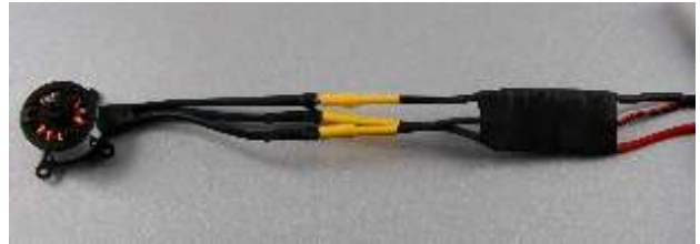
21. Connect the motor and ESC , Pls make sure the motor running direction is correct , if not , pls discretionarily exchange any two wires of the three Wires .
