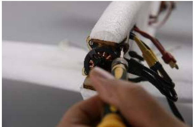
22. Tighten the motor by using the screws which included into the motor bag.
