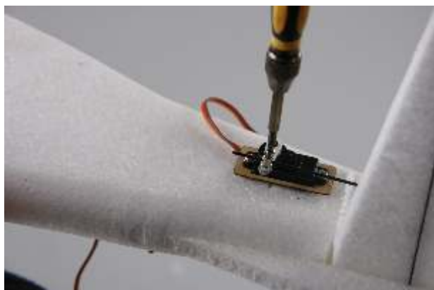
20. Install the rudder servo, horn and pushrod, the method is same as installing elevator servo, horn and pushrod .
