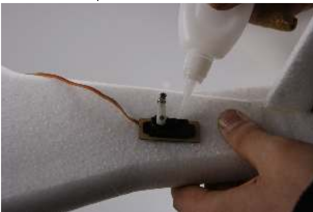
15. Glue the servo mount into the servo hole of the fuselage by using CA.
