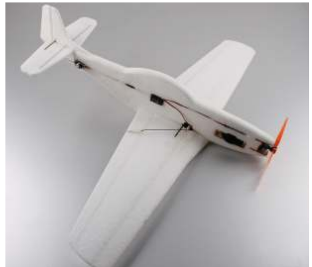
27. Use a O-ring to fix the propeller .
