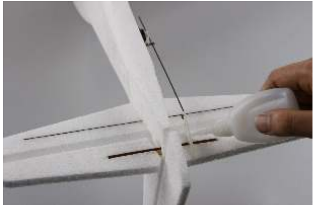
17. Install the elevator horn and pushrod , the method is same as installing aileron horn and pushrod .
