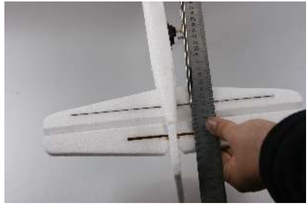
16. Use a knife to cut a elevator servo slot
