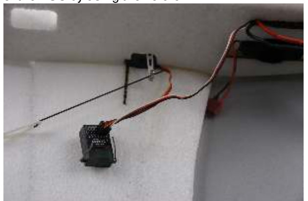
24. Install the ESC plug and servo wire plug into the receiver slot , and then debug.
