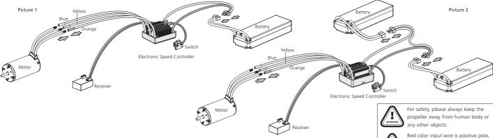
1) Picture 1 is for Seaking-30A-V3, Seaking-60A-V3 and other ESCs that work with one LiPo battery pack; that is a wiring diagram with 1 battery pack. 2) Picture 2 is for Seaking-120A-V3, Seaking-180A-V3, Seaking-130A-HV-V3 and other ESCs that may work with two LiPo battery packs; that is the wiring diagram with 2 battery packs. Black color input wire is negative
