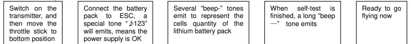
Please note that we use a special way to represent the cells quantity of a lithium battery pack: 1 long “beep—” = 5 short “beep-”. For example, 2 long “beep—” plus 2 short “beep-” (Beep—Beep—BB) means a 12 cells lithium battery pack, 1 long “beep—” plus 1 short “beep-” (Beep—B) means a 6 cells lithium battery pack, and so on.
