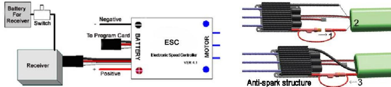
**Note:** There are 2 control wires on the HV controller. The longer one is close to the positive battery wire, which is connected with the receiver, and the shorter one is close to the negative battery wire, which is used to connect the program card to set the programmable parameters of the controller.
