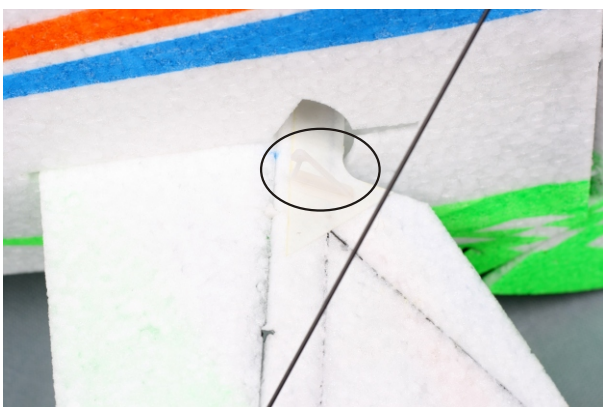
24. Install the elevator control horn.
