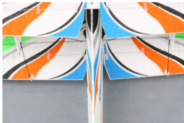
34. Install the aileron control linkage, using the same techniques that you used to install the aileron pushrod.
