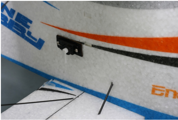
25. Install the rudder control horn.
