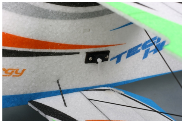
22. Install the elevator servo and the rudder servo into the servo mount.
