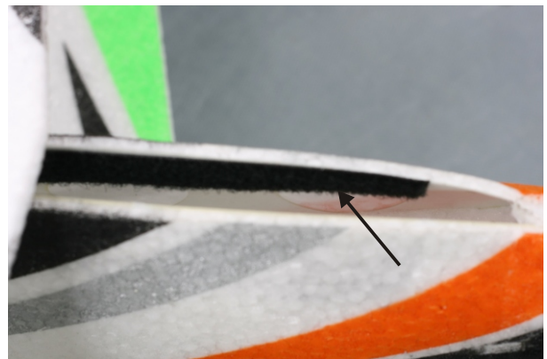
39. Cut 1pcs velcro, then fix them inside the cockpit as shown in above picture.
