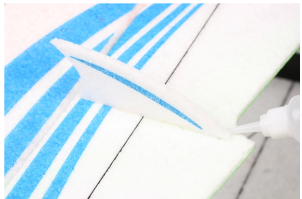
37. Glue the wing fences to the wing. Make sure they are vertical.
