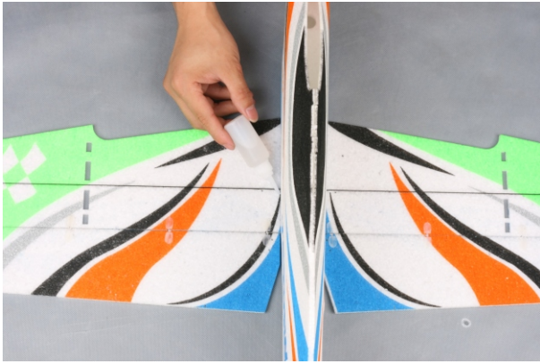
7. Key the bottom wing into the fuselage. Center the wing and glue it to the fuselage.
