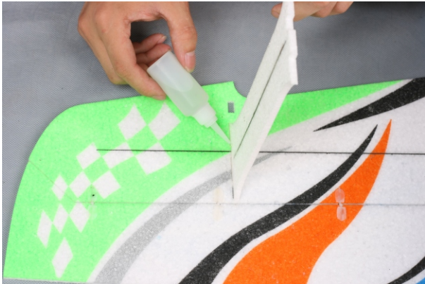
8. Glue the two wing struts to the bottom wing.
